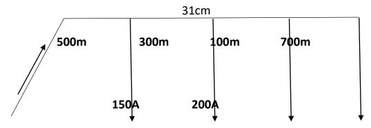
The single line diagram of distributer with its topped current.
