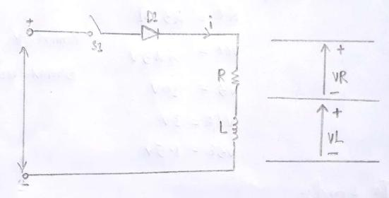
⇒ when SI is closed at t=0, the current throug the Inductor Increases and is expressed as:
