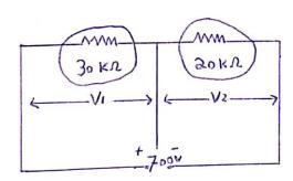
voltage divides rule, the readings of the two voltmeter are:
