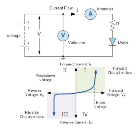
The I-V Characteristic Curves for a silicon diode are non-linear and very different to that of the previous resistors linear I-V curves as their electrical characteristics are different. Current-Voltage characteristics curves can be used to plot the operation of any electrical or electronic component from resistors, to amplifiers, to semiconductors and solar cells.
