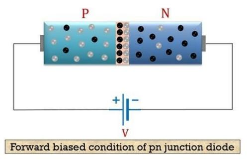
So, when forward biasing is provided to the device as shown above. Then the majority carriers from both sides, i.e., holes from p side and electrons from n side experience a repulsive force from the positive and negative terminal of the battery respectively.
