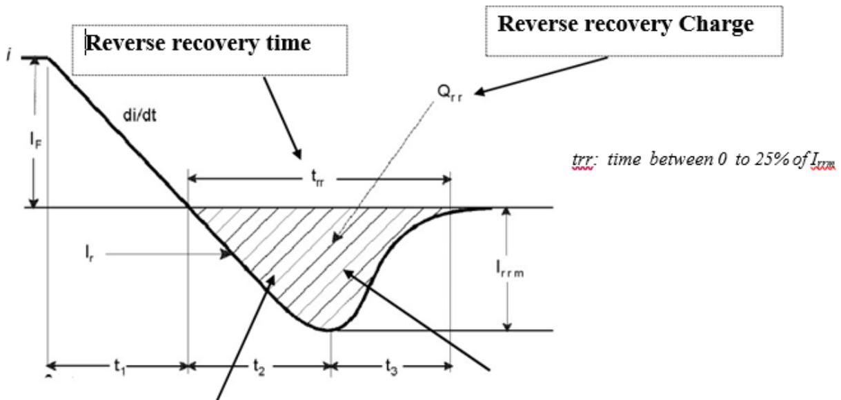
*Due to the minority carriers, which remain stored in the pn-junction (depletion region), and represents the time between zero crossing and the peak reverse current,  $I_{rrm}$ .*
