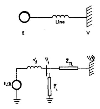
Swing equation provides the equation of motion of the rotor of the finite machine and it require development of expressions for the mechanical and the electrical powers
