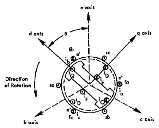
Define the *d* axis of the rotor at some instant of time to be at angle  $\Theta$  radians with respect to a fixed reference position and project the stator phase currents ia, iband ic, (currents leaving the generator terminals) along the d and *q* axes of the rotor
