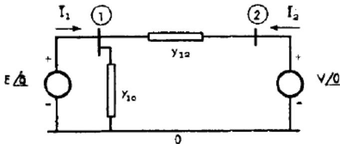
$$\begin{bmatrix} \bar{I}_1 \\ \bar{I}_2 \end{bmatrix} = \begin{bmatrix} \bar{Y}_{11} & \bar{Y}_{12} \\ \bar{Y}_{21} & \bar{Y}_{22} \end{bmatrix} \begin{bmatrix} \bar{E} \\ \bar{V} \end{bmatrix}$$
