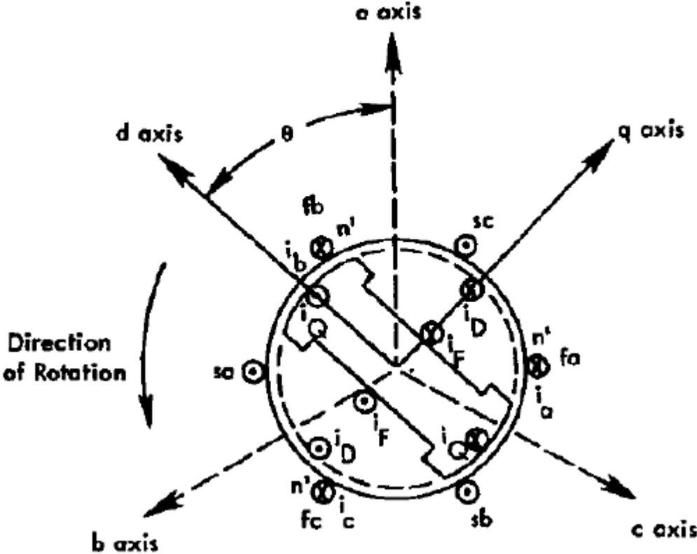
Define the *d* axis of the rotor at some instant of time to be at angle  $\Theta$  radians with respect to a fixed reference position and project the stator phase currents  $i_a, i_b$  and  $i_c$ , (currents leaving the generator terminals) along the *d* and *q* axes of the rotor
