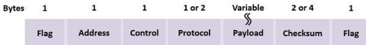
Frame format for PPP protocol
