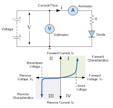
The I-V Characteristic Curves for a silicon diode are non-linear and very different to that of the previous resistors linear I-V curves as their electrical characteristics are different. Current-Voltage characteristics curves can be used to plot the operation of any electrical or electronic component from resistors, to amplifiers, to semiconductors and solar cells.
