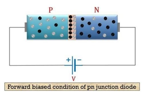
the representation of forward biasing applied to a PN junction diode:
