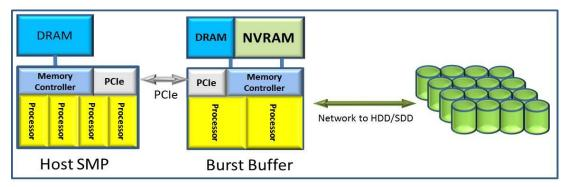
A tier of solid-state burst buffers is integrated into the storage system to absorb application I/O requests. This storage system is designed for use by large-scale HPC (high performance systems). Enhancements to the CODES of storage system simulator are done to enable burst buffer simulations.
