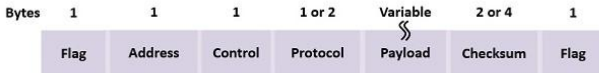
Frame format for PPP protocol
