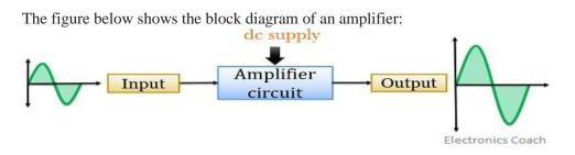
Here, as we can see the transmitted signal is fed to the amplifier as input. The circuitry involved inside the amplifier raises the amplitude of the signal up to the desired level and then further transmits it to the receiver.
