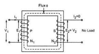
The primary draws a current  $I_1$  which is just necessary to produce flux in the core. As it is magnetizing the core, it is called magnetizing current denoted as  $I_u$ . As the transformer is ideal, the winding reactance is zero and it is purely inductive in nature. The magnetizing current is very small and lags  $V_1$  by 30° as the winding is purely inductive. This  $I_u$  produces an alternating flux  $\Phi$  which is in phase with  $I_u$ .
