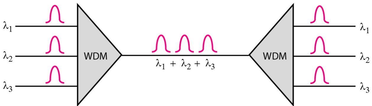
The following Figure is Prisms in WDM multiplexing and demultiplexing
