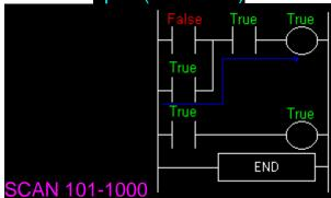
Notice that even when the low level sensor is false there is still a path of true logic from left to right. This is why we used an internal relay. Relay 1000 is latching the output(500) on. It will stay this way until there is no true logic path from left to right.(i.e. when 0001 becomes false)
