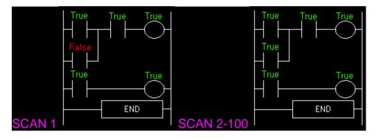
Gradually the tank fills because 500(fill motor) is on.
