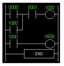
Let's watch what happens in this program scan by scan. Initially the tank is empty. Therefore, input 0000 is TRUE and input 0001 is also TRUE.
