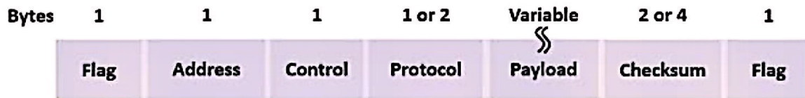
Frame format for PPP protocol
