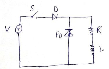
When The Switch is closed a steady Current will flow Through the load. When we open the Sevitch the Current will Start To decay. This decay of Current Will result in development of Vollage across the Torminals of inductor due te this voltage The free Wheeling diode mill be porcoord bias and it will ad like
