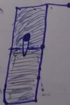
Shearing failure edge of plate -
