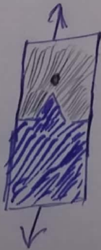
Transverse tension failure
