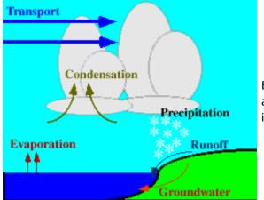
Evaporation of warm surface water increases the amount of moisture in the colder, drier air flowing immediately above the lake surface. With continued evaporation, water vapor in the cold air condenses to form ice-crystal clouds, which are transported toward shore.
