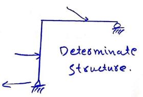
Mathematically speaking, in a determinant Structure the total number of reaction and Member forces required to be Calculated are equal to or less than the number of eq. of static equilibrium and available.
