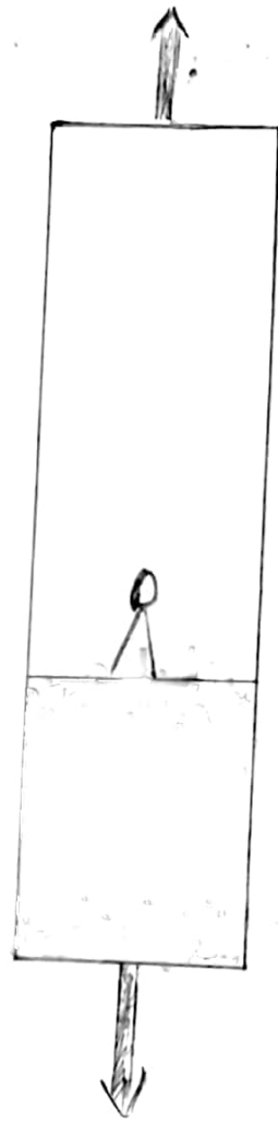
Transverse Tension failure.
