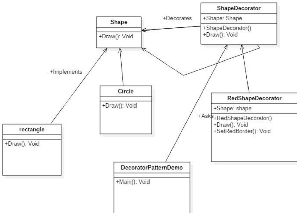
**Q5: Design Pattern 10 Marks** Suppose we have the following java files. Identify the pattern also Considering the java files draw class diagram?
