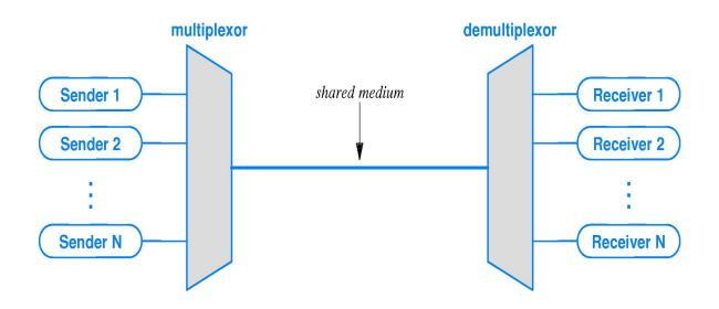
Figure 11.1 The concept of multiplexing in which independent pairs of senders and receivers share a transmission medium.
