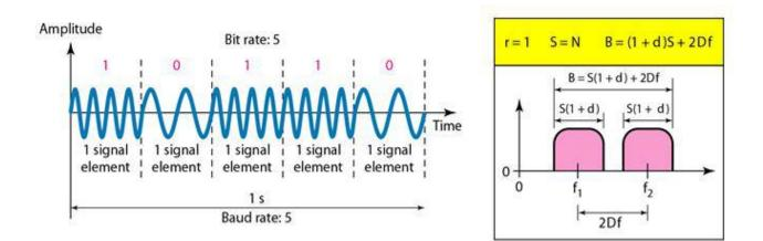
The above figure shows, the middle of one bandwidth is f1 and the middle of the other is f2. Both f1 and f2 are  $\Delta f$  apart from the midpoint between the two bands. The difference between the two frequencies is  $2\Delta f$ .
