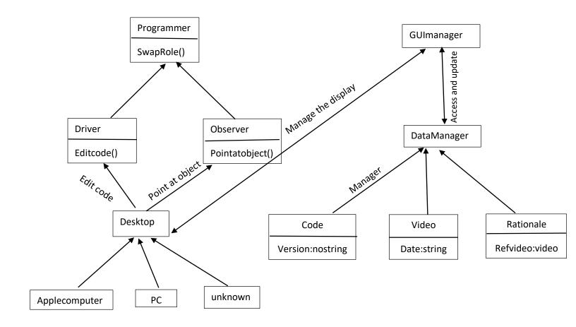
The sample class diagram above captures most of the classes and relationships. I have inserted an UnknownDesktop class for future extension of RPP. Obviously when I designed this class diagram I already have the AbstractaFactory design pattern in my mind.
