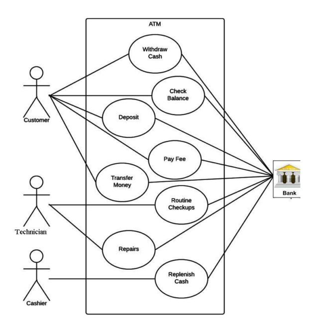
A use case diagram at its simplest is a representation of a user's interaction with the system that shows the relationship between the user and the different use cases in which the user is involved. Basically it shows how a user interacts with the system and the bank
