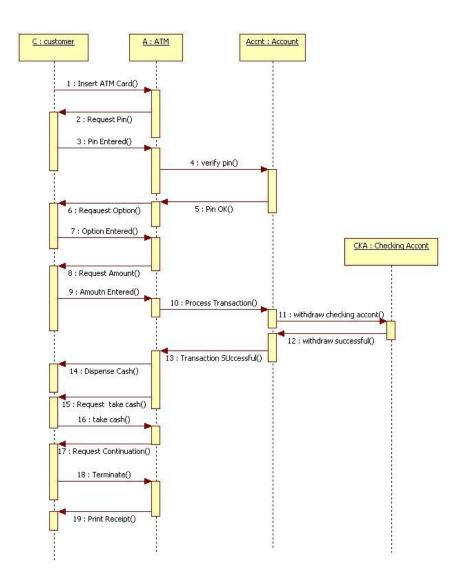
A sequence diagram shows object interactions arranged in time sequence. the objects and classes involved in the scenario and the sequence of messages exchanged between the objects needed to carry out the functionality of the scenario. This is basically depends on exchange of messages with eachother.
