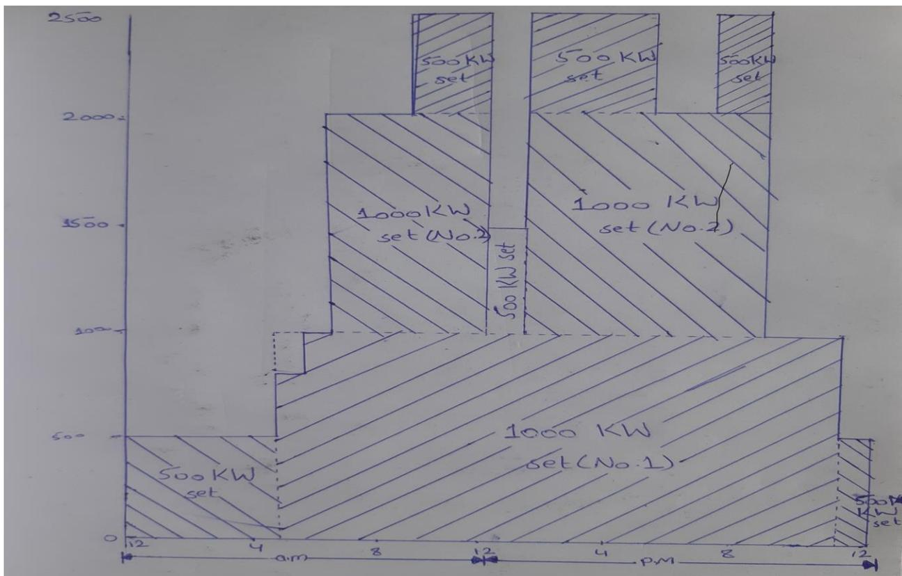
From the load curve we can see that **three generator sets will suffice** with the following ratings
