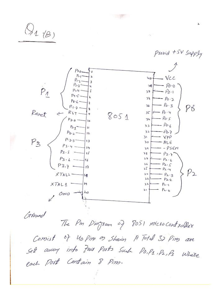
3 Que # 01 (c) Auswer :-The Pin Configuration of 8057 is exactly Similar to that Sosi except That the First two Points P1.0 and P1.1 are multiplexed to correspond to Times 2 operation as given in following Table. Existing Alternate Function. input P1.0 T2 Times 2 External count P1.1 T2Ex Times 2 Trigger input. input So 8052 also hay Times 22. & Past D) Answed :-
