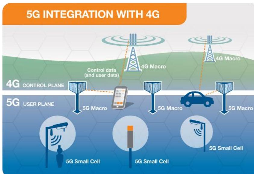
When a 5G connection is established, the User Equipment (or device) will connect to both the 4G network to provide the control signaling and to the 5G network to help provide the fast data connection by adding to the existing 4G capacity. Where there is limited 5G coverage, the data is carried on the 4G network providing the continuous connection. Essentially with this design, the 5G network is complementing the existing 4G network
