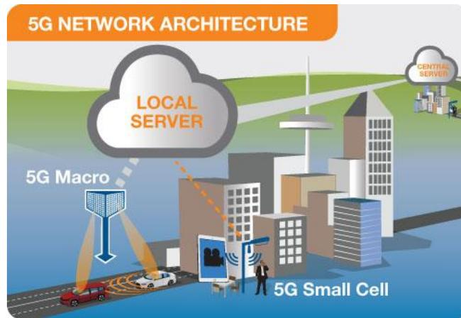
Example of a local server in a 5G network providing faster connection and lower response times
