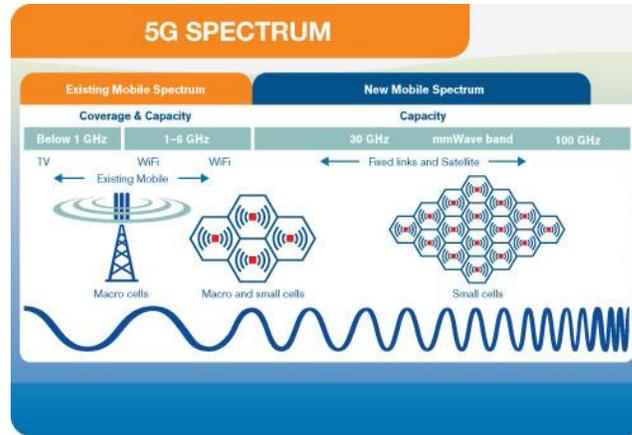
Mobile spectrum showing the radio frequency range from 3-100 GHz with new 5G spectrum above 6GHz.
