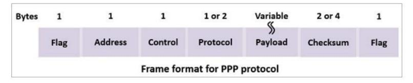
The PPP frame contains two flag fields, a protocol filed to determine the Type of packet residing in the payload, and a payload field which can Variety. However, the rest of the fields are the same as the HDLC protocol.
