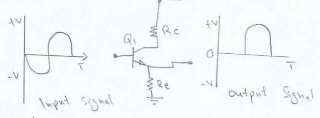
It is clear from the circuit that the base of the transistor Q1 is not biased and the rive half cycle of waveform is missing in output. It improves Power efficiency it creates a lot of distortion
