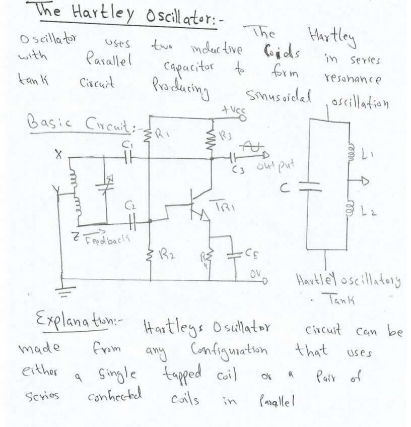
when the circuit is oscillating the voltage at Point X (collector), relative to Point X emitter is 180° out - of - Phase with the voltage at Point Z(base) velative to Point y
