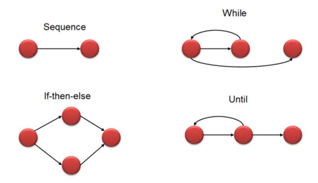
Consider three software items: Program-X, Control Flow Diagram of Program-Y and Control Flow Diagram of Program-Z as shown below
