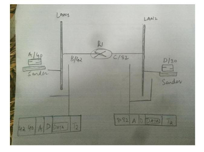
Assume that the communication is between a process running at computer A with port address *i* and a process running at computer D with port address *j*. Show the contents of the Packets and Frames at the network, data link and transport layer for each hop interface.
