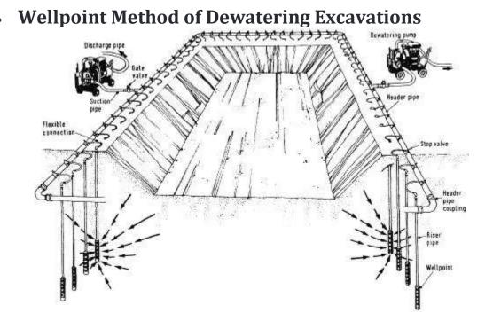
1) A series of wells of required depth are created in the vicinity of the excavated area from where the water has to be pumped out. The wells are arranged either in a line or a rectangular form where the wellpoints are created at a distance of at least 2m from each other.
