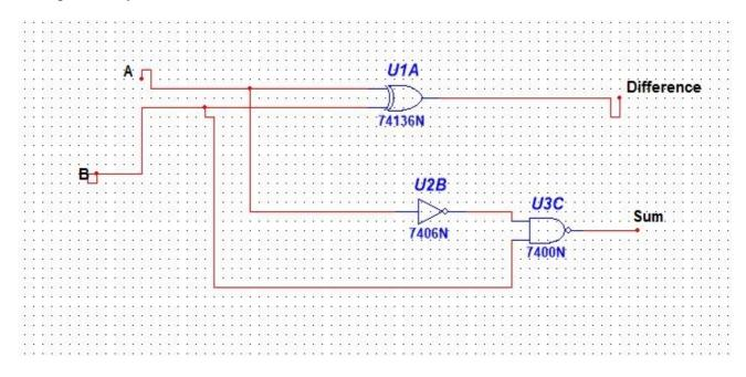
If we monitor cautiously, it is fairly clear that the variety of operation executed by this circuit which is accurately related to the EX-OR gate operation. Therefore, we can simply use the EX-OR gate for making difference. In the same way, the borrow produced by half adder circuit can be simply attained by using the blend of logic gates like AND- gate and NOT-gate.
