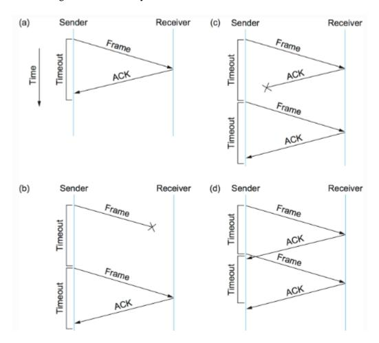
Referring to the diagram above, it can be explained that one way to ensure reliable transmission is the *stop-and-wait* algorithm. The idea of stop-and-wait is straightforward: After transmitting one frame, the sender waits for an acknowledgment before transmitting the next frame. If the acknowledgment does not arrive after a certain period of time, the sender times out and retransmits the original frame.
