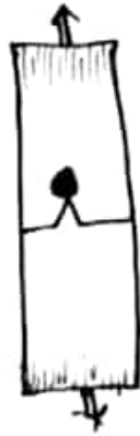
Transverse Tension failure.
