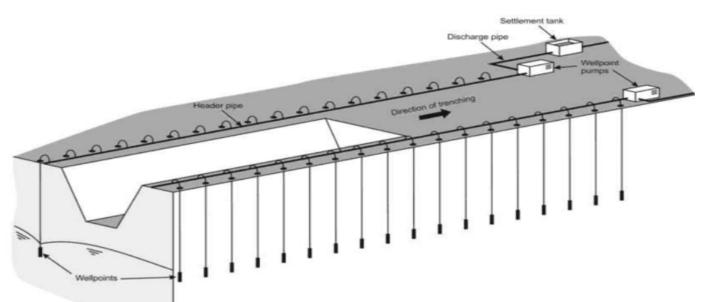
spacing (1 to 3 m centres) around the excavation. • Commonly used for dewatering of pipeline trenches • Can be a very flexible and effective method of dewatering in sands or sands and gravels • Drawdown limited to 5 or 6 m below level of pump due to suction lift limits • Individual wellpoints may need to be carefully adjusted ("trimming").
