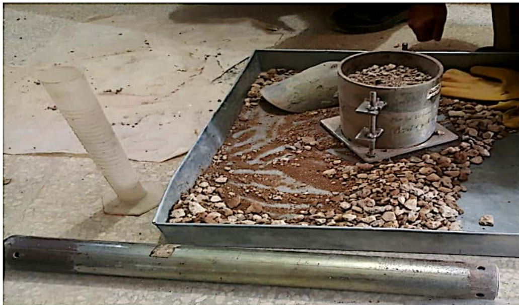
Figure 4.2.CBR mould for sample preparation.
