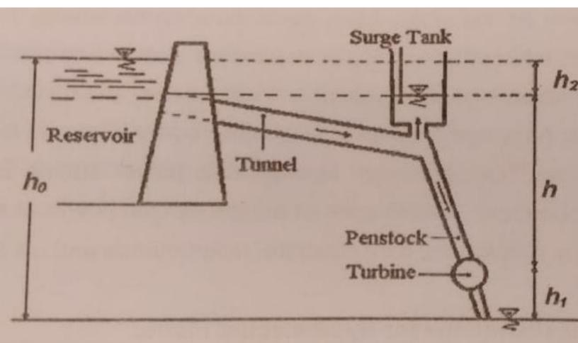
A hydroelectric plant consists of a reservoir for storage of water, a diversion dam, an intake structure for controlling and regulating the flow of water, a conduit system to carry the water from the intake to the waterwheel, the turbines coupled with generators, the draft tube for conveying water from waterwheel to the tailrace, the tailrace and a power house i.e., the building to contain the turbines, generators, the accessories and other miscellaneous items.
