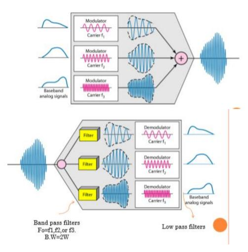
BLOCK DIAGRAM OF FDM DEMULTIPLEXING
