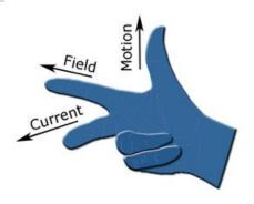
This effect is a result of **FARADAYS LAWS OF ELECTRO MAGNETIC INDUCTION** (i.e. when the conductor moves through a magnetic field, it generates an electric field perpendicular to the magnetic field & direction of conductor). The induced EMF is given by
