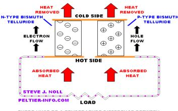
THERE MUST BE A TEMPERATURE DIFFERENCE BETWEEN THE HOT AND COLD SIDES FOR POWER TO BE GENERATED
