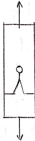
transverse tension failure
