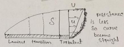
Fig show the relocity distribution in turbulent boundary layer shows a much steeper gradient near wall and flatter through out reming layer.
