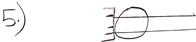
Electrical Outlet — 5 Amps.
