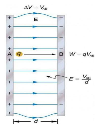
The work done by the electric field in Figure 1 to move a positive charge q from A, the positive plate, higher potential, to B, the negative plate, lower potential, is
