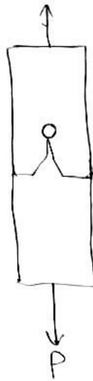
Transverse tension failure.
