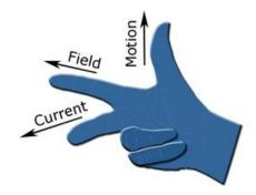
This effect is a result of FARADAYS LAWS OF ELECTRO MAGNETIC INDUCTION. (i.e. when the conductor moves through a magnetic field, it generates an electric field perpendicular to the magnetic field & direction of conductor). The induced EMF is given by
