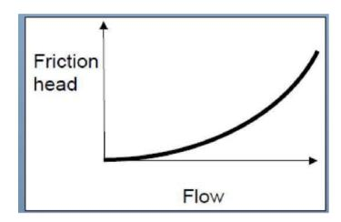
System Head is the sum of static head and friction head
