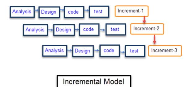
The system is put into production when the first increment is delivered. The first increment is often a core product where the basic requirements are addressed, and supplementary features are added in the next increments. Once the core product is analyzed by the client, there is plan development for the next increment.
