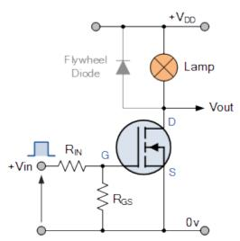
In this circuit arrangement an Enhancement-mode N-channel MOSFET is being used to switch a simple lamp "ON" and "OFF" (could also be an LED).
