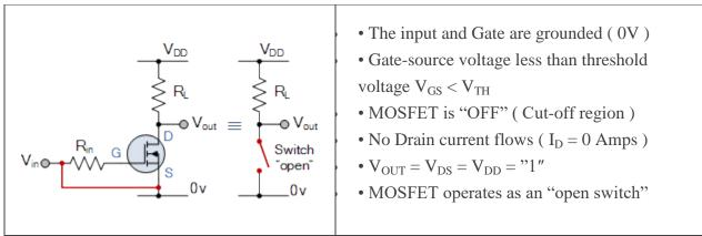
Then we can define the cut-off region or "OFF mode" when using an e-MOSFET as a switch as being, gate voltage,  $V_{GS} < V_{TH}$  thus  $I_D = 0$ . For a P-channel enhancement MOSFET, the Gate potential must be more positive with respect to the Source.
