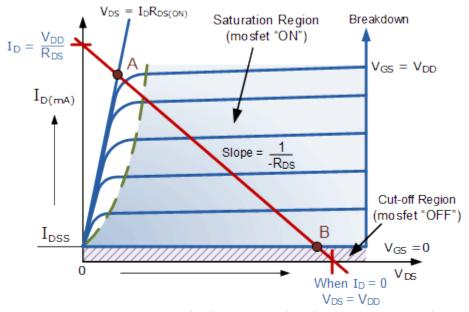
The minimum ON-state gate voltage required to ensure that the MOSFET remains "ON" when carrying the selected drain current can be determined from the V-I transfer curves above. When  $V_{IN}$  is HIGH or equal to  $V_{DD}$ , the MOSFET Q-point moves to point A along the load line.
