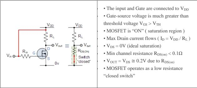
Then we can define the saturation region or "ON mode" when using an e-MOSFET as a switch as gate-source voltage,  $V_{GS} > V_{TH}$  thus  $I_D$  = Maximum. For a P-channel enhancement MOSFET, the Gate potential must be more negative with respect to the Source.
